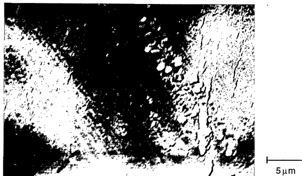
Figure 5.5: SEM-picture of a plasma modified membrane at 100 W and 60 min.
